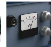
Our screwdrivers are tested for dielectric strength under a 10,000 volt load to make sure that their most important property, their insulation, has been exhaustively tested. Each individual Wera VDE screwdriver is subjected to this
